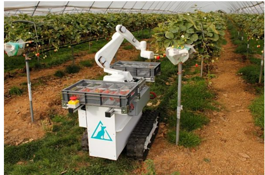
Autonomous robot to harvest soft fruits Dogtooth Technologies
